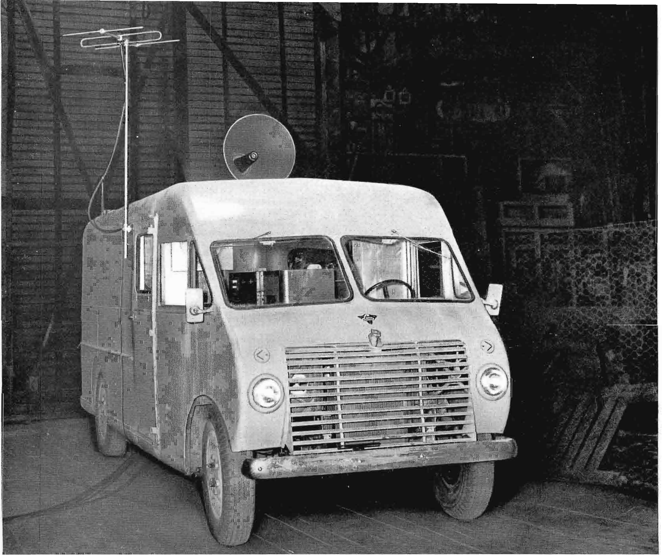
FIG. 1. The new mobile unit shown above, developed by the RCA International Division, carries all the technical equipment usually found in a radio studio control room. The picture shows the unit with the VHF transmitting antenna and the public address horn mounted ready for use.
