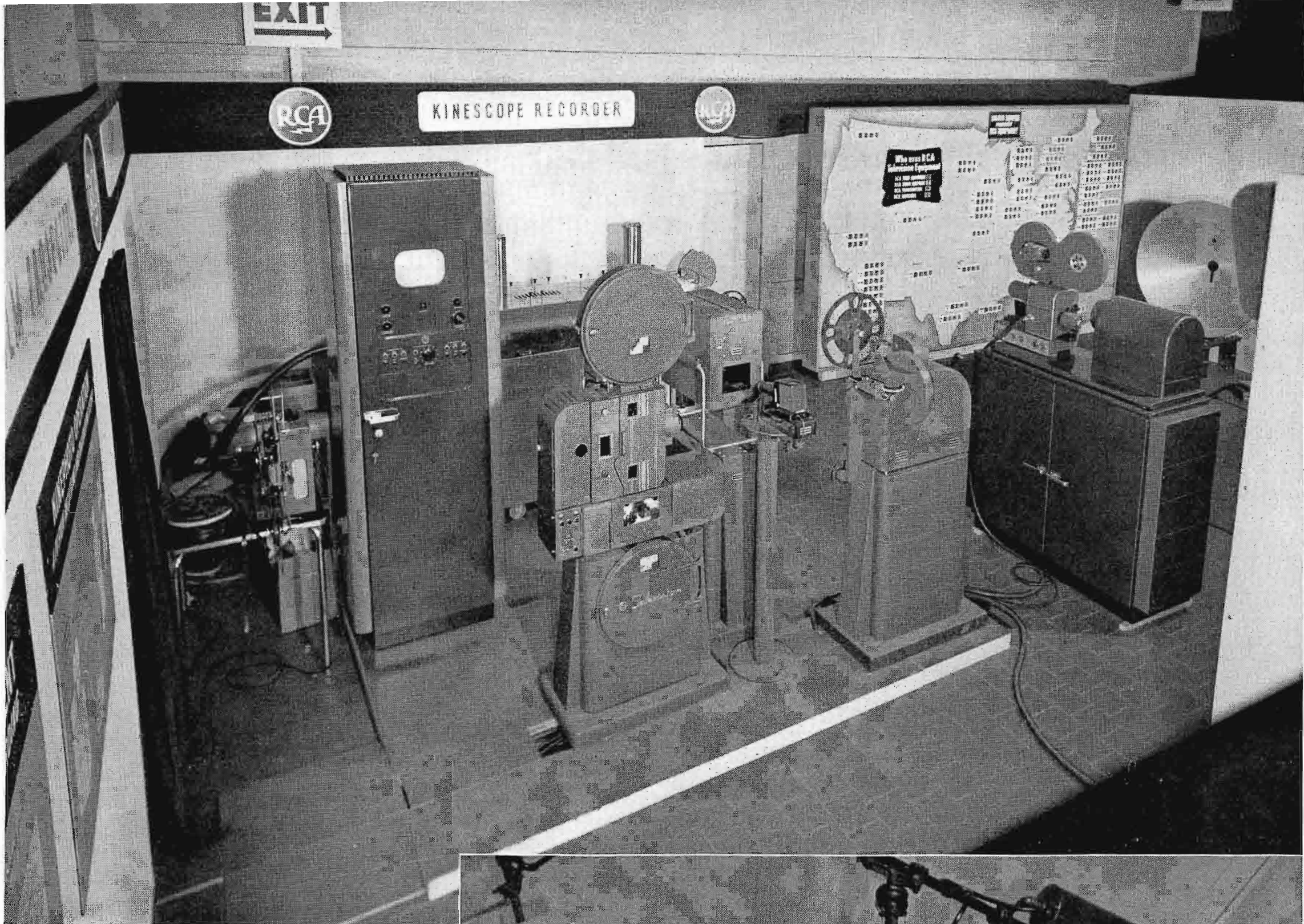
FIG. 7 (above). This is the TV film equipment area. At left is the monitoring and power supply rack, in center foreground the 35mm and 16mm projectors (with film camera between). At the right is the kinescope recorder.
