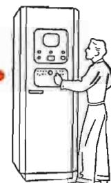
RCA Film Camera Monitor Rack. This is the control center of the projection room. It houses the amplifiers, all necessary rack-mounted power supplies, and the kinescope for viewing the film pictures.
