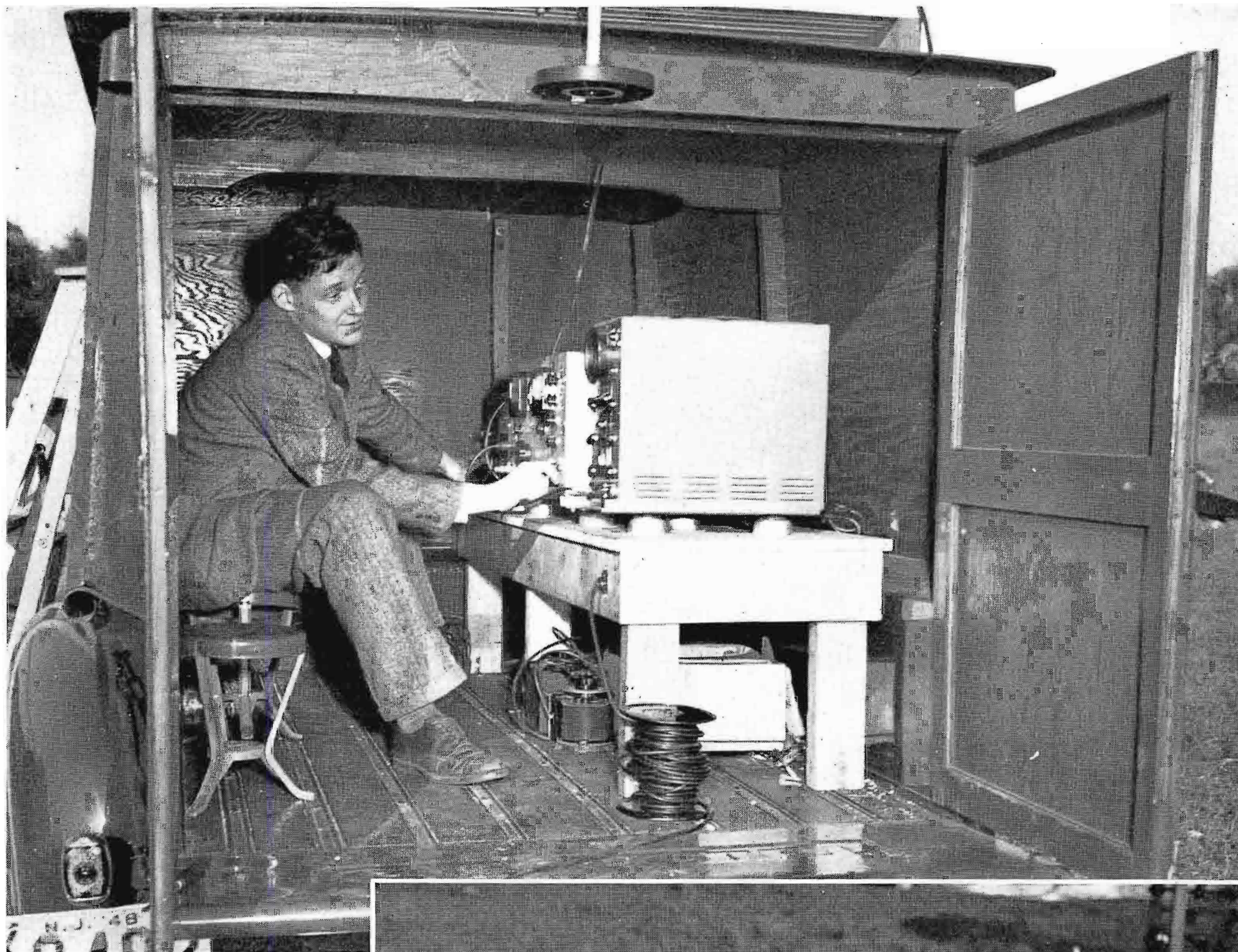
FIG. 4. Photo above shows E. M. Brown, co-author, at the controls of the receiving equipment mounted in a Chevrolet truck with a plywood enclosure. Wheel at top of the picture controls antenna rotation.
