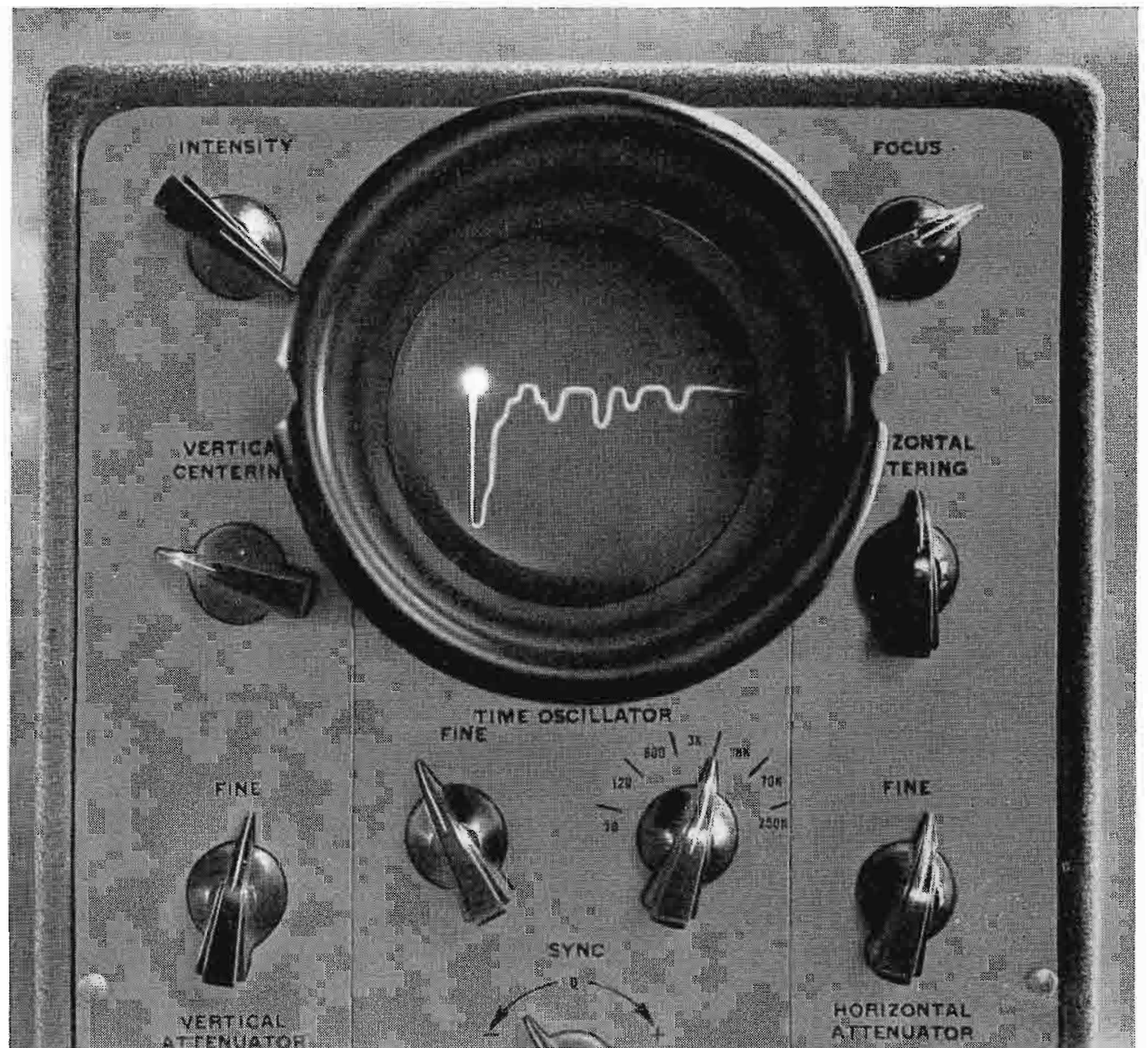
FIG. 10. This photo of the oscilloscope was taken under conditions of severe multi-path reception. The main pulse (negative polarity) is shown directly below the bright dot. Note that first echo occurs during the decay time of the main pulse. This echo alone would account for distorted picture on television receivers in the home.
